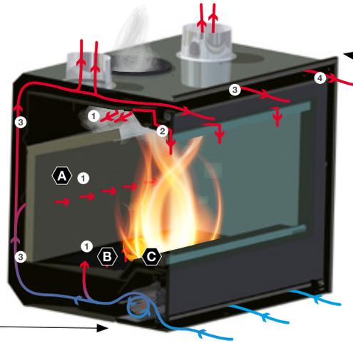
A - Vermiculite / Neotherm inside / B - Cast iron grate / C - Big ash draw
